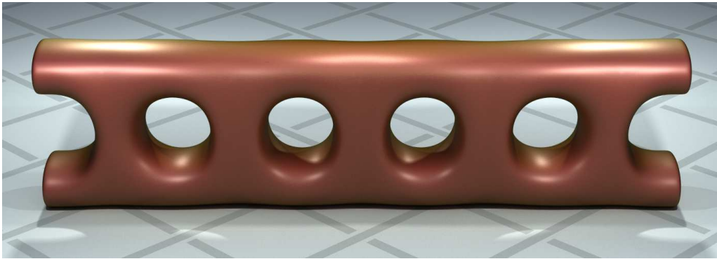
Fig. 5.4 – Another layer of simple_glossy_bsdf with sharper highlights is added with weighted_layer .
